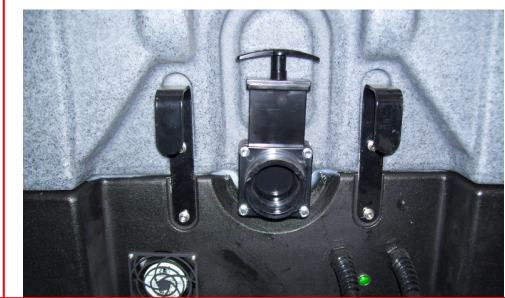
Remove four bolts holding valve assembly to flange fitting
