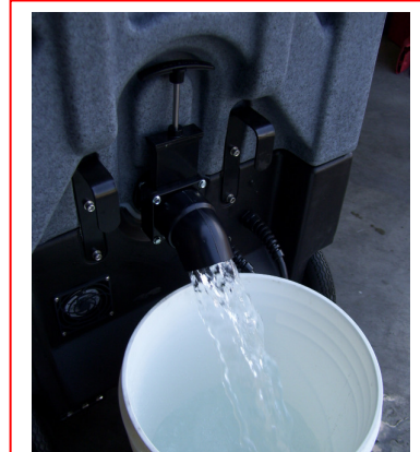
Vacuum acid solution out of Solution Tank
